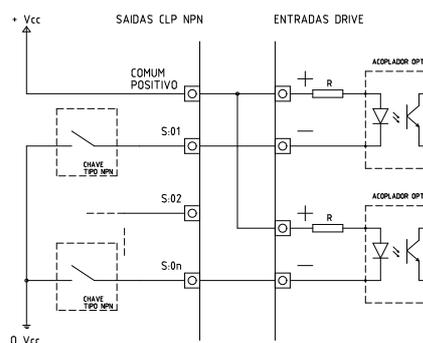
**Figura 18:** Interface com circuito NPN
