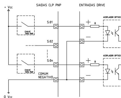
**Figura 17:** Interface com circuito PNP
